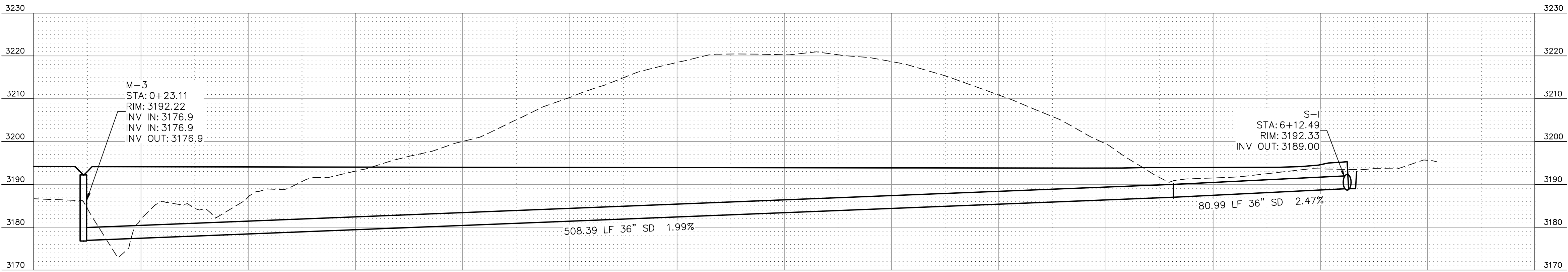
SOUTHEAST DRAINAGE CULVERT PROFILE
